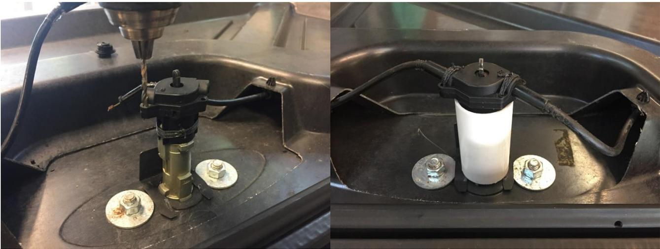
Grab a piece of scrap PVC pipe, slot it, and cover up lock cylinder.
