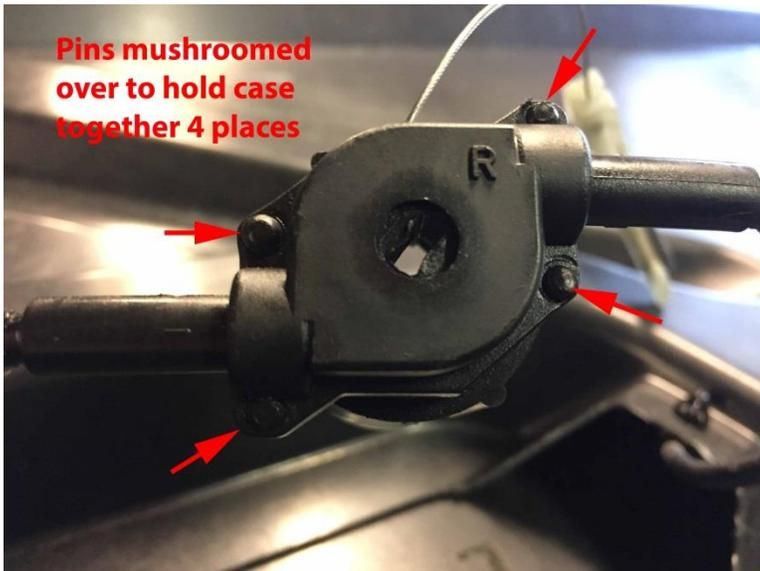
You can slice off these pins and open the case so you can see what is shown in the first picture.
