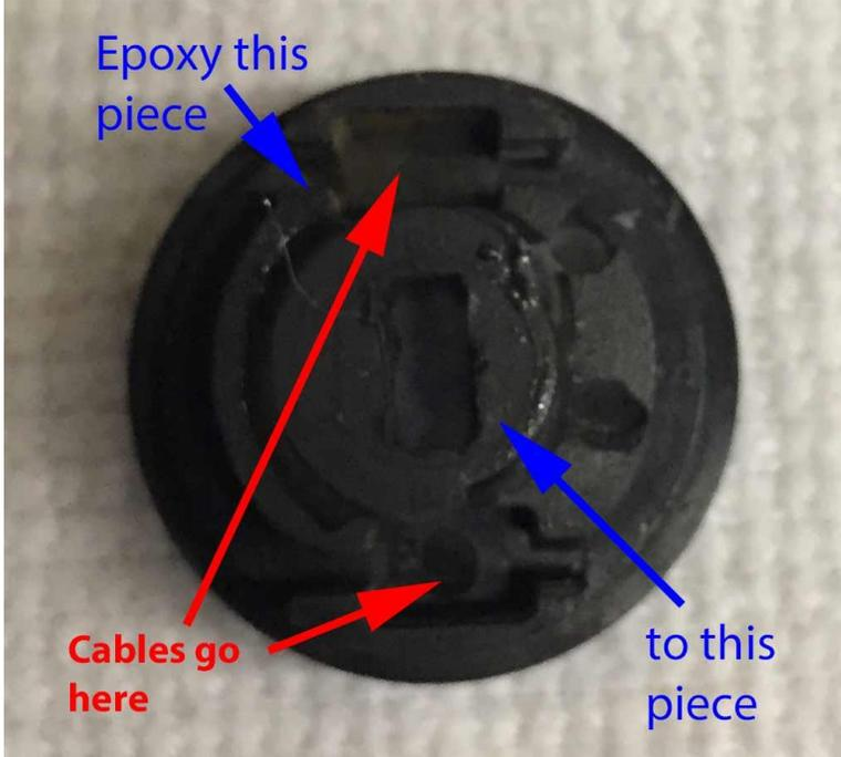
Reassemble the case, using heavy thread or archery serving along with some epoxy. You may have to shave the pins a bit or open up the top holes with a drill to get them to fit back together.
