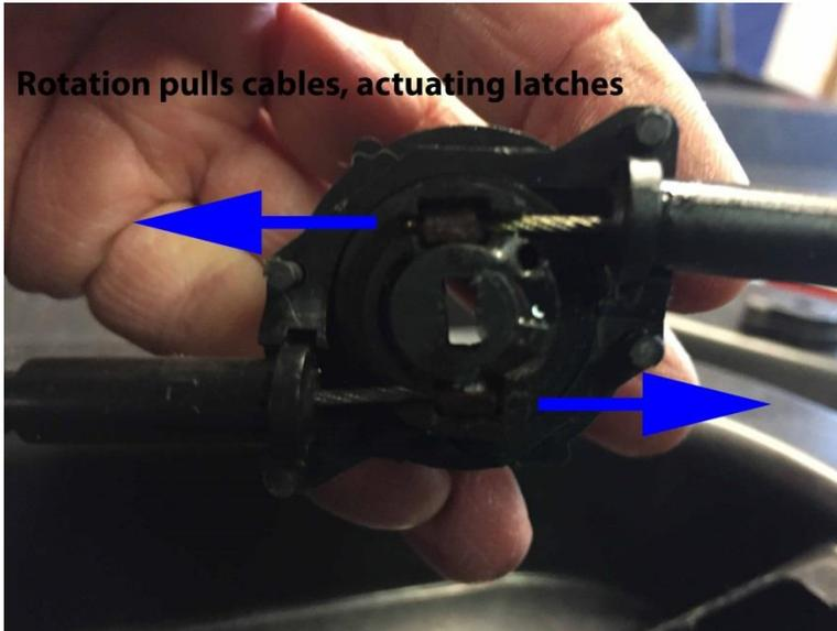
It is easy to disassemble the top from the case, it is held together by 4 pins that are mushroomed over:
