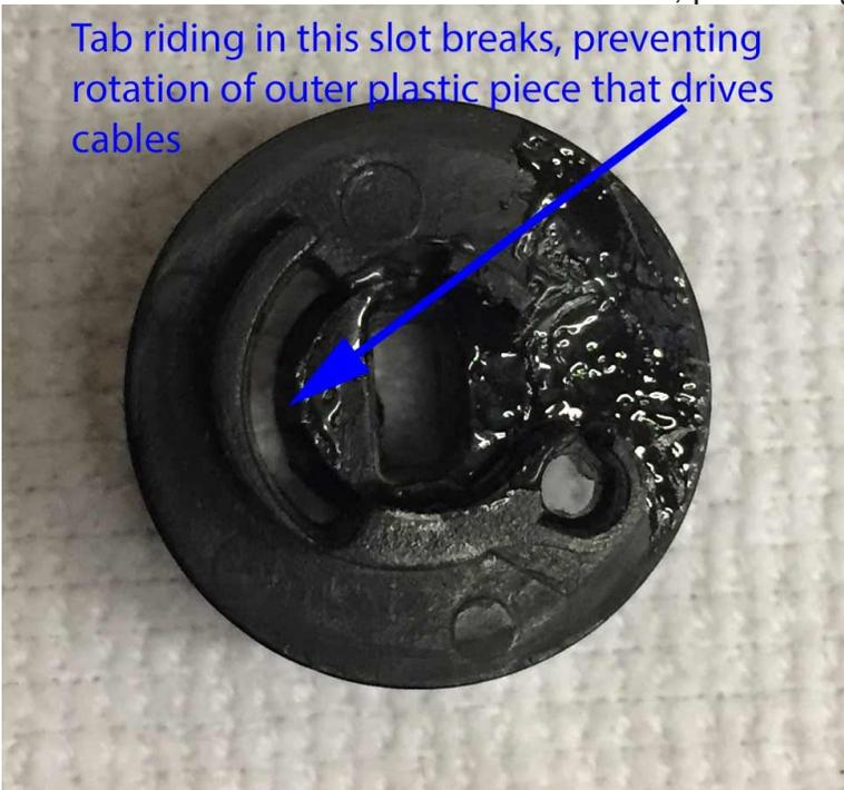
The solution is to epoxy these two discs together so that the keyway actuates the cables. Keep the inner disc keyway orientation in reference to the cable pockets as shown here.
